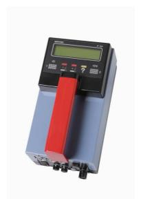
The IF104 is a hand-held device which processes and displays the data measured by a SHF, SHI or SEC probe (see the corresponding leaflet). The  $\gamma$  dose rate measurement can be performed from 1  $\mu$ Gy/h to 300 Gy/h with these probes.
